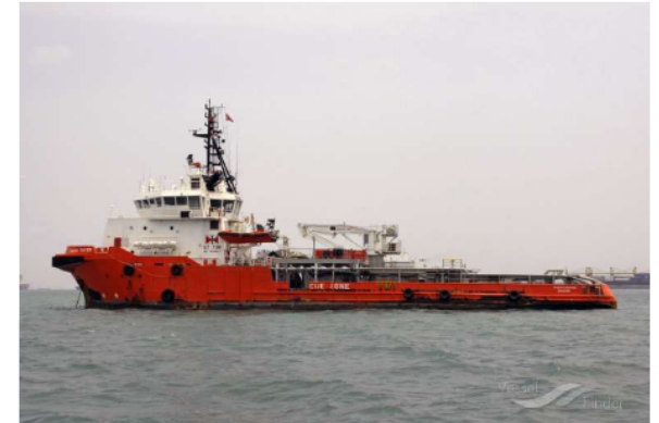
Name: M.V. Mahanadi Type: 80 Ton AHTSV Build: November 2006 Country of Origin: Indonesia
